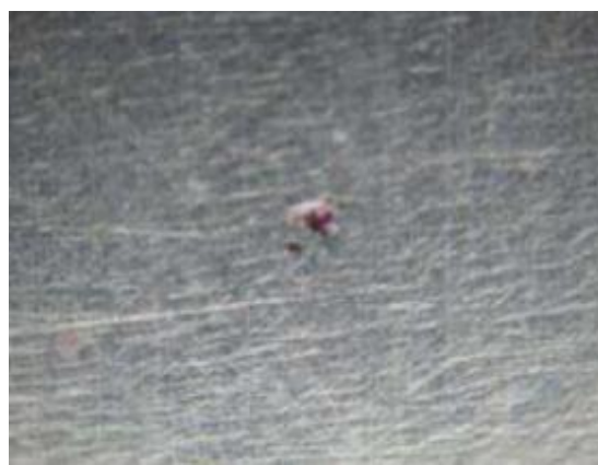
Fig. 1. Small hole or pore in stainless steel caused by pitting corrosion.
