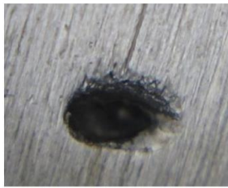
Fig. 1 Cavities in which microorganisms (biofilm) can develop
